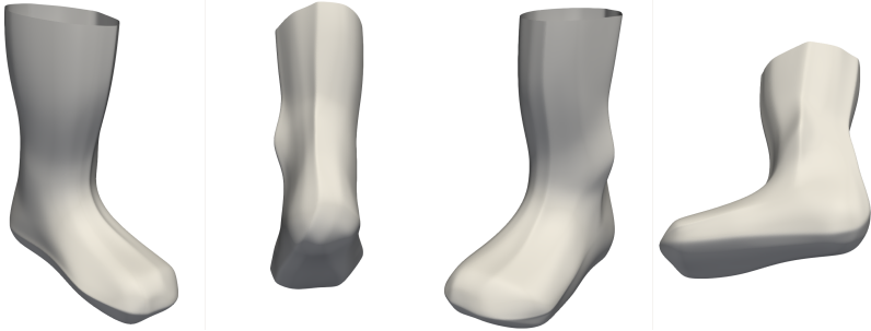
Figure 3.3: Once a SDF is available it can be queried on a voxel grid to recover an arbitrary amount of points on the manifold p \in \Omega(t) at \phi_t(p) = 0 . Marching cubes algorithm then yields a polygonal surface mesh which is depicted here.
