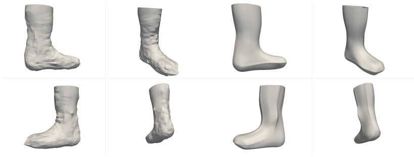
Figure 3.11: Side-by-side comparison of reconstructions from the linear regression model ( left ) and the implicit neural representation ( right ). The resolution of the implicit neural representation reconstruction is chosen extremely fine at the cost of considerable computational overhead.
