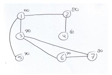
An example of a network with seven nodes. Next to each node is the current battery level (so node 3 has level 90 left). Nodes are neighbors if they are connected, so node 1 and 2 are each others neighbors, but 3 and 4 are not.
