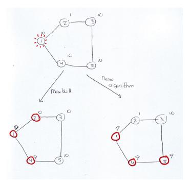
With MaxWill this network is down after sending one message from node 1, because its neighbors 2 and 4 have to relay the message to reach all two-hop neighbors. So node 2 will immediately run out of battery. In the new algorithm, nodes 4 and 5 relay the message and it is possible to send at least one more message.
