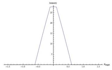
For the example cup suggested by Philips the intensity became a nice and simple peek.
