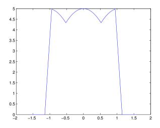
For a cup with slightly different inclined edges the intensity pattern was something like a batman mask. This is the torch light effect.
