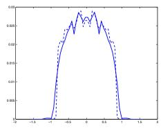
The results from the first method on a smooth cup (solid line). The preliminary sample contained 512 rays, the estimation sample  $2^{18}$ . They compared the pattern with the naive ray-tracing of  $2^{18}$  rays (dashed line).
