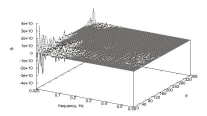
At the first try the least squares method found a solution with negative values. This might theoretically be the best solution for the given data, but in reality the response of the ship cannot be negative. Therefore a constrained least Squares method was used that only returns positive solutions.
