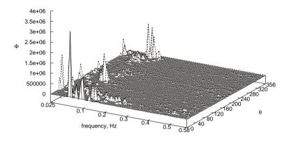
The resulting solution was very, very spiky. For a small change in the frequency or angle of the incoming wave, there would suddenly be a very strong reaction from the vessel. But the actual relation has to be smooth; changing the waves a bit should only change the reaction of the ship a bit.
