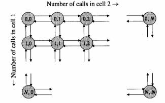
Figure 7.2: State space for the two-base-station system. N denotes the maximum number of calls accepted in a cell
