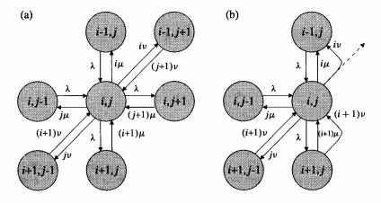
Figure 7.4: Transitions and transition rates with mobility, (a) for a state in the interior of the state space and (b) for a state on the boundary of the state space
